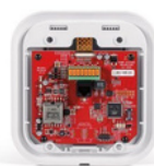
Tesira TEC-1i. Panel de control remoto
